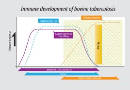
BIONOTE BTB Ab ELISA 2.0 detects mid to late (anergy) stage of TB affected cattle by antibody titer check againt TB (Laboratory method for antibody check)
